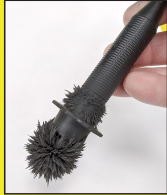
Magnetic wand covered in powder. Note the bristle-effect.
